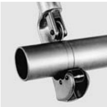
Fig. 1 Cutting the pylon
