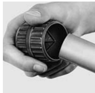
Fig. 2 Deburring the cut edge
